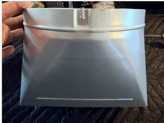
PHOTO 2 Supplied rectangle-to-8" round transition
